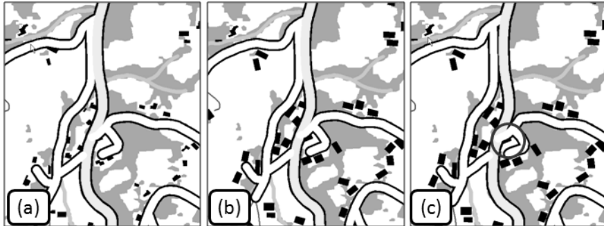
Figure 12: (a) initial rural area. (b) rural space generalised by CartACom. (c) Roads generalised by the Beams with a side effect on the circled building.
