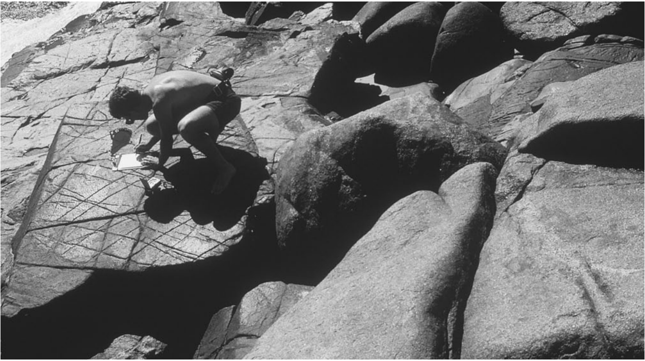
FIGURE 6.1 A geologist measuring fractures in an outcrop, near Tuross Point on the southeastern coast of Australia. The more intensely fractured rock is a fine-grained mafic intrusive and the less fractured rock is a coarse-grained felsic intrusive.
