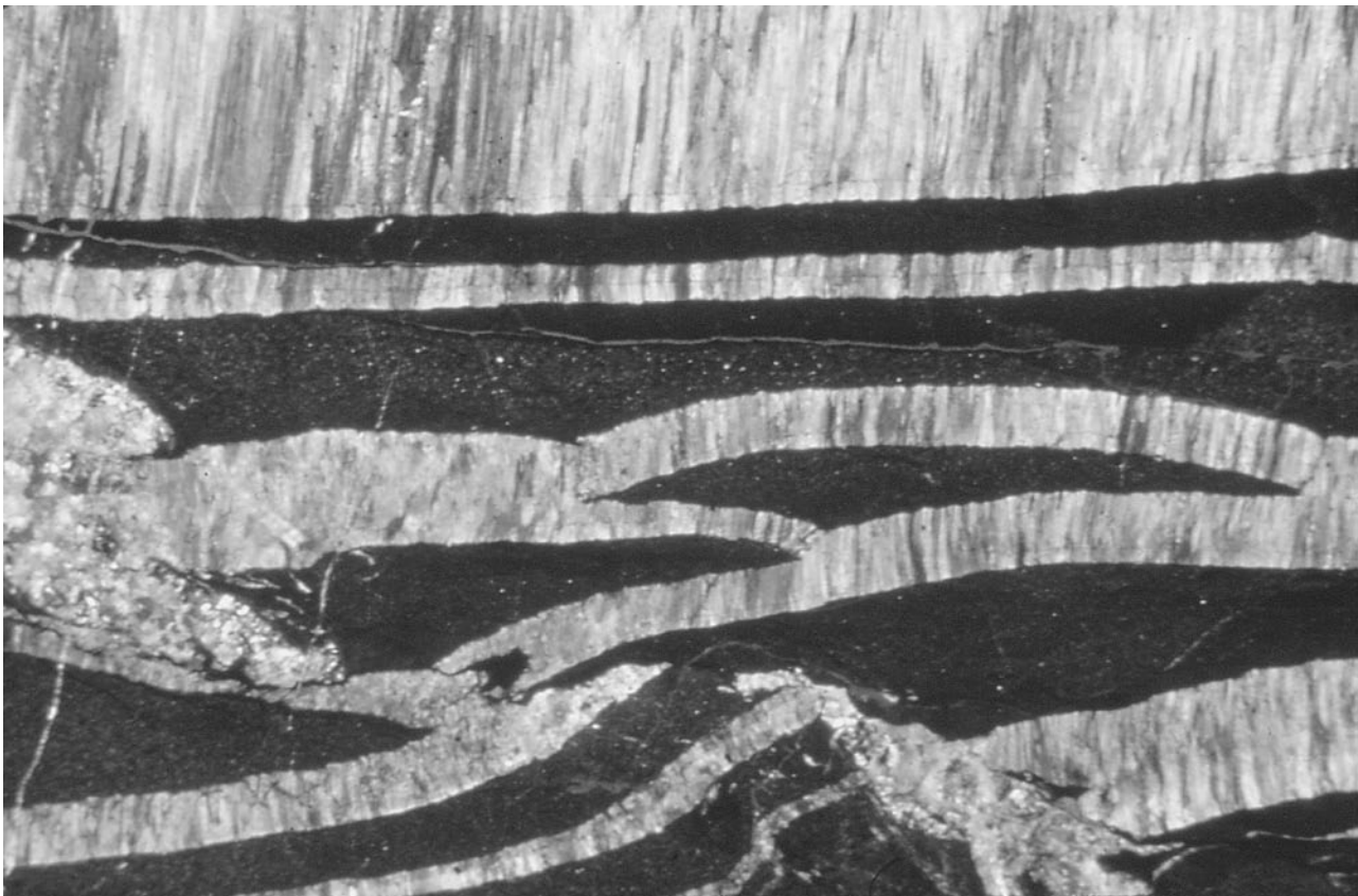
FIGURE 7.25 Photomicrograph of fibrous calcite filling in tensile fractures. Width of view is ~3 cm.
