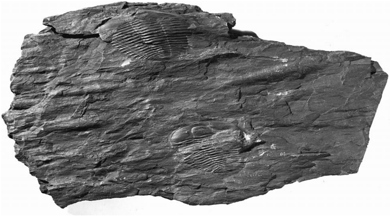
FIGURE 4.1 Deformed trilobites ( Angelina sedgwicki ) in a Cambrian slate from Wales. Knowledge about their original symmetry enables us to quantify the strain.
