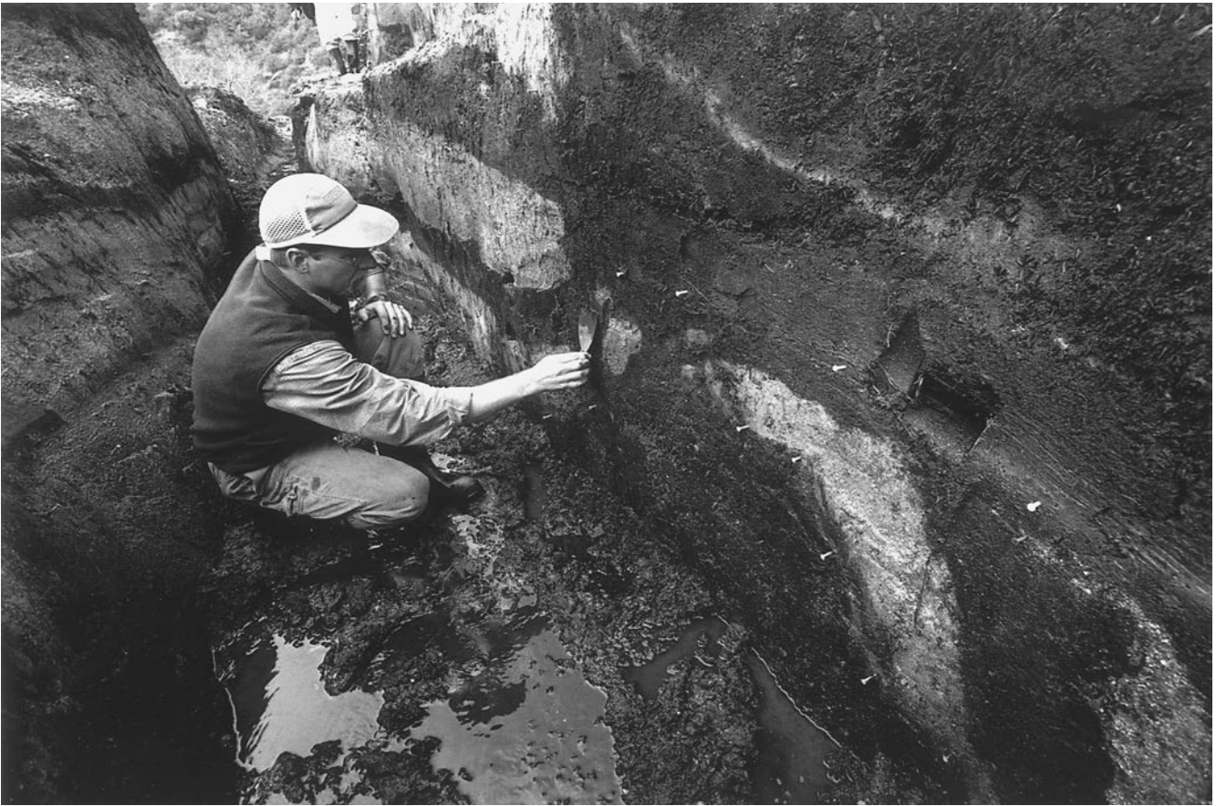
FIGURE 8.37 Nearly horizontal layers of light-colored rock and gravel, and dark-colored peat have been broken and distorted as a result of earthquake activity near Banning, California, along the San Andrea Fault.
