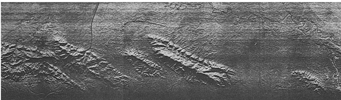
FIGURE 19.13 A side-scan radar image from the Darien Basin in eastern Panama showing an array of en echelon anticlines whose formation has arched up the land surface, creating a set of ridges. The field of view is about 50 km. Note that the geometry of these structures indicates left-lateral shear.
