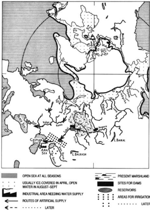
Fig. 113 Scheme for reversal of the flow of the Russian and Siberian rivers, the Pechora, Ob and Yenesei, to water the arid lands in Soviet central Asia.
